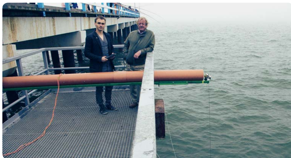
Figure 12: Prototype of a linear wave generator attached to a pier in Palanga, Lithuania (picture: Klaipeda University Coastal Research and Planning Institute)
