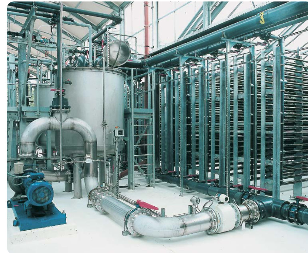
Figure 13: Photobioreactor for the production of green algae (picture: IGV GmbH)
