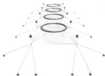
Figure 3. Basic diagrams showing cage farms. The structure consists of an anchoring arrangement, a floating structure and a net cage.
