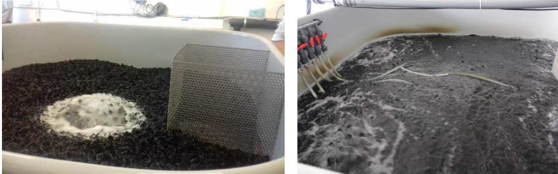
Figure 6. Biological filtration - a moving bed - preparation (1) and working (2). Photo: T.Kulikowski/NMFRI
