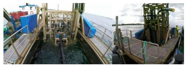
Figure 17: Harvest of a net farm (Musholm), using a UW harvester.
