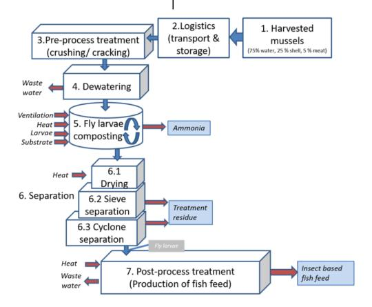
Figure 22. Insect process line flowchart
